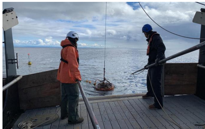
Figure 4. ESP at surface waiting to be lifted onto the deck. A total of 76 eDNA samples were autonomously collected in 2024. Image Credit: John Micket, UW-APL
