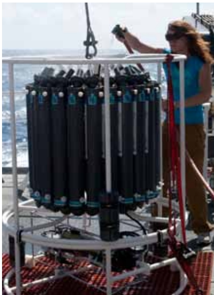
A CTD with water sampling bottles attached to the rosette frame. Image courtesy of NOAA Okeanos Explorer Program.
