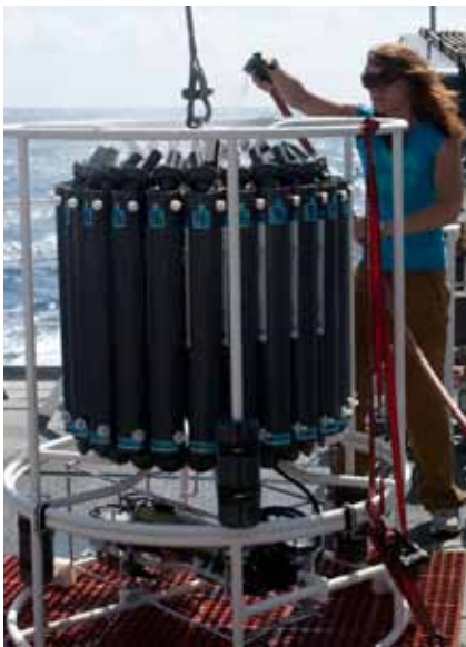
A CTD with water sampling bottles attached to the rosette frame. Image courtesy of NOAA Okeanos Explorer Program.
