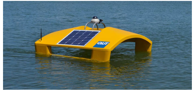
Figure 3. One of the ASVs from the Inference system. The navigation sensors, computing, and batteries are located underneath the two solar panels. The scientific payload, in this study the GGS described in Section 3.2.2, is attached to the moon-pool opening underneath the camera.
