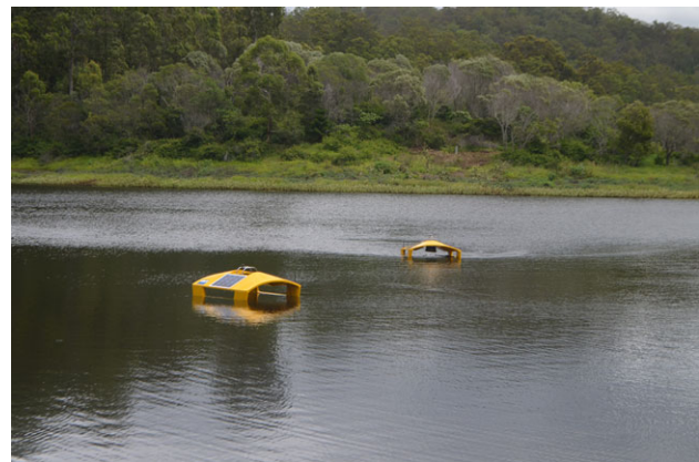
Figure 12. Two Inference ASVs fitted with GSSs during testing in South East Queensland. The retracted gas sampling unit is visible underneath the ASV on the right.
