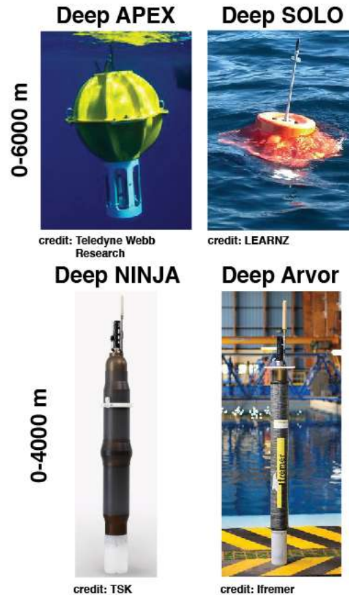
Figure 1: The four Deep Argo float models: the Deep APEX floats, developed by the University of Washington and Teledyne Webb, the Deep SOLO floats, developed by Scripps Institution of Oceanography, the Deep NINJA floats, developed by Japan Agency for Marine-Earth Science and Technology (JAMSTEC) and Tsurumi-Seiki Co. (TSK), and the Deep Arvor floats, developed by Institut Français de Recherche pour l'Exploitation de la Mer (Ifremer), Centre national de la recherche scientifique (CNRS), and nke instrumentation.
