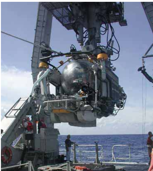
Launching the Johnson-Sea-Link II submersible from the R/V Seward Johnson .
