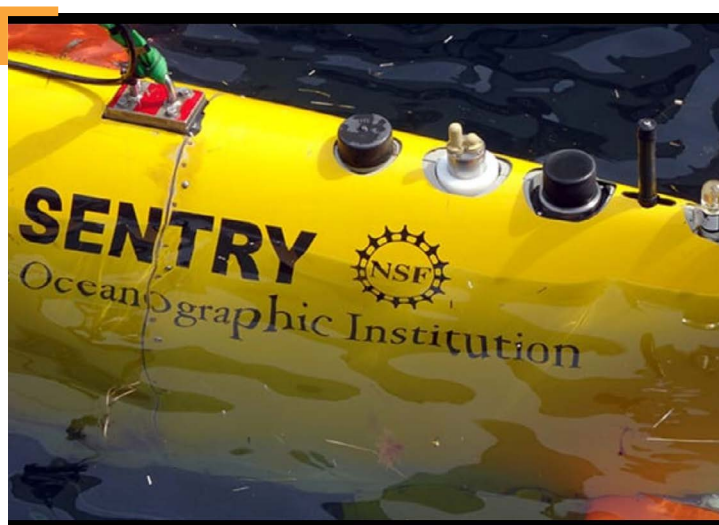
A variety of communication and tracking devices line the top of Sentry , allowing scientists to stay in continuous touch with the AUV. Photo by Richard Pittenger, Woods Hole Oceanographic Institution. https://www.whoi.edu/multimedia/a-sentry-in-the-sea/
