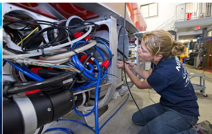
A WHOI engineer installs a new shroud over one of the maneuvering thrusters on the Nereid Under-Ice remotely operated vehicle. Photo by Tom Kleindinst, Woods Hole Oceanographic Institution. https://www.whoi.edu/multimedia/under-the-ice/
