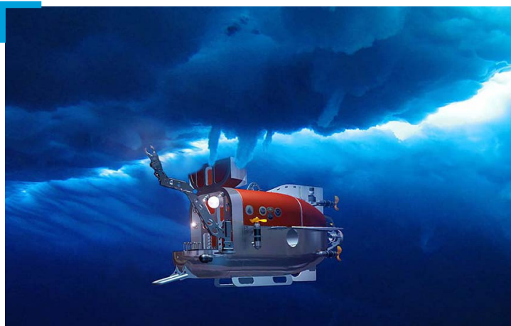
Nereid Under-Ice , a hybrid remotely operated vehicle designed and built by researchers in WHOI's Deep Submergence Laboratory. Illustration by Casey Machado, Woods Hole Oceanographic Institution. https://www.whoi.edu/multimedia/nereid-under-ice/
