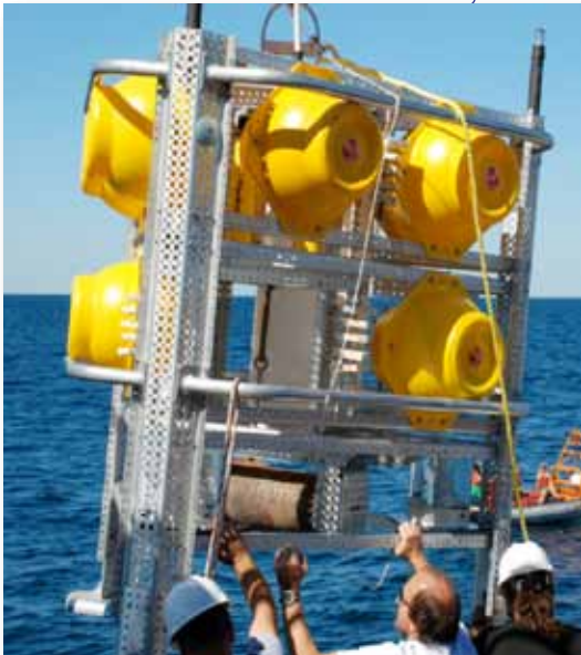
Benthic landers, designed at the University of North Carolina – Wilmington, will be used during Deepwater Mid-Atlantic Canyons Project. They provide a way to deploy multiple instruments and experiments to the deep-sea floor and collect precise time-series data on environmental variability that is typically unattainable. Image courtesy SW Ross, UNC-W. http://oceanexplorer.noaa.gov/explorations/11midatlantic/hires/plan_fig6_hires.jpg
