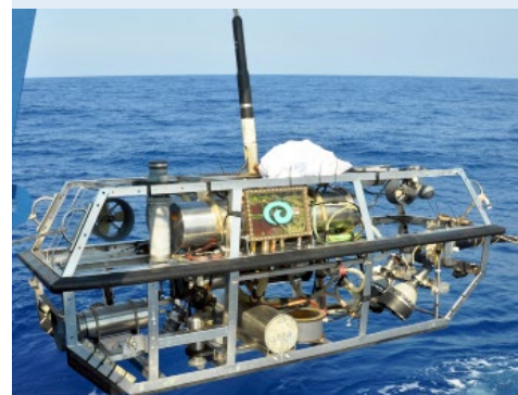
Argus (right) acts as a stabilizing platform for Hercules , following the ROV into the water. Image courtesy of The Ocean Exploration Trust. http://oceanexplorer.noaa.gov/technology/subs/hercules/argus.html
