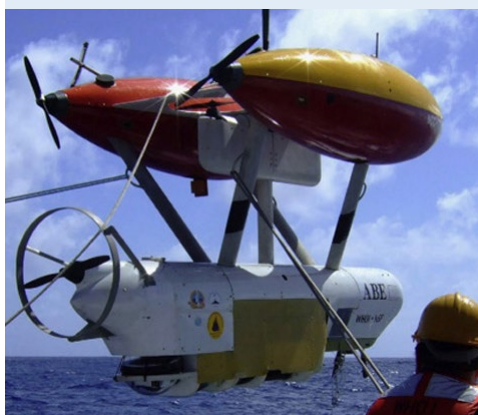
The autonomous benthic explorer (ABE) a free-swimming robot, was used on multiple expeditions to find new hydrothermal vents in the deep ocean all over the world, from New Zealand to South Africa and Brazil to Ecuador. Photo courtesy of Christopher German. http://oceanexplorer.noaa.gov/explorations/10chile/background/exploration/media/exploration1.html
