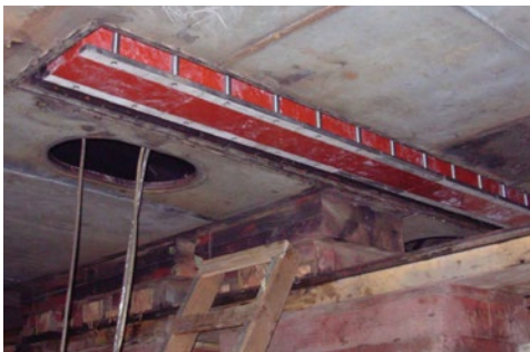
One of the EM302 transducers installed on the hull of the NOAA Ship Okeanos Explorer in 2008. Image courtesy of NOAA OER. http://oceanexplorer.noaa.gov/okeanos/explorations/ex1503/logs/jun6/media/em302.html
