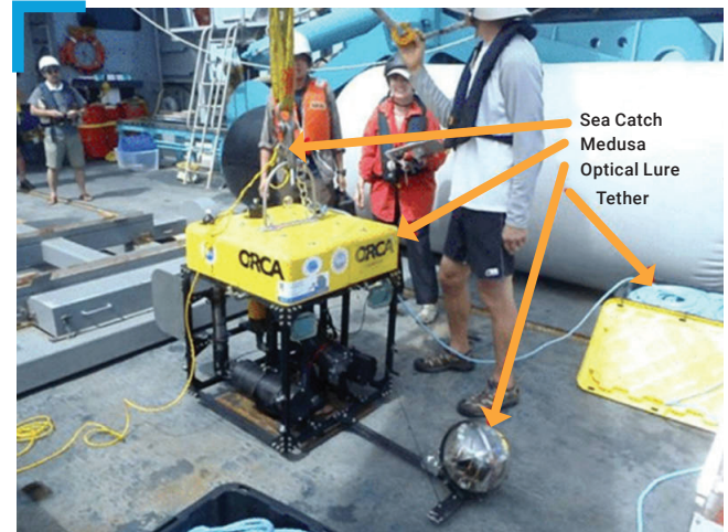
The Medusa camera system with optical lure and cable tether. Image courtesy of NOAA Ocean Exploration.
